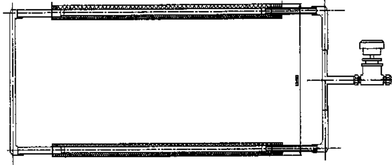
Figure 16. Flat loop thermosyphon made from polymer composite (Polyamide reinforced by carbon nine filaments and nano diamond particles)
