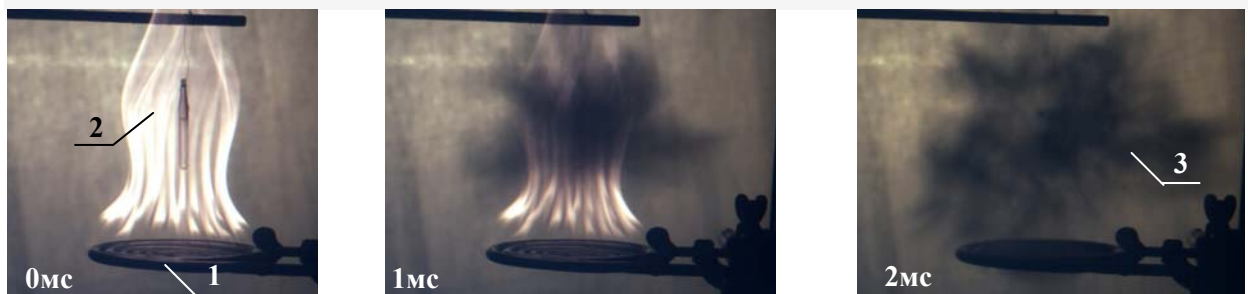
Fig8. Quenching the flame of the spiral (diameter \sim 10\text{ cm} ) gas burner by DW cloud of steam explosion of cylindrical glass capsule ( L = 45\text{mm} , d = 5\text{ mm} , \Delta = 0.5\text{ mm} , V = 0.25\text{ml} ), placed in a burner flame. 1 – spiral burner, 2 - burner flame, 3 - DW cloud, formed by the explosion of the capsule.
