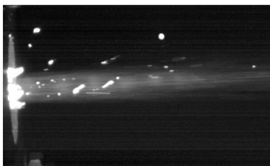
Fig. 6. Spraying process in a supersonic plasma jet.
