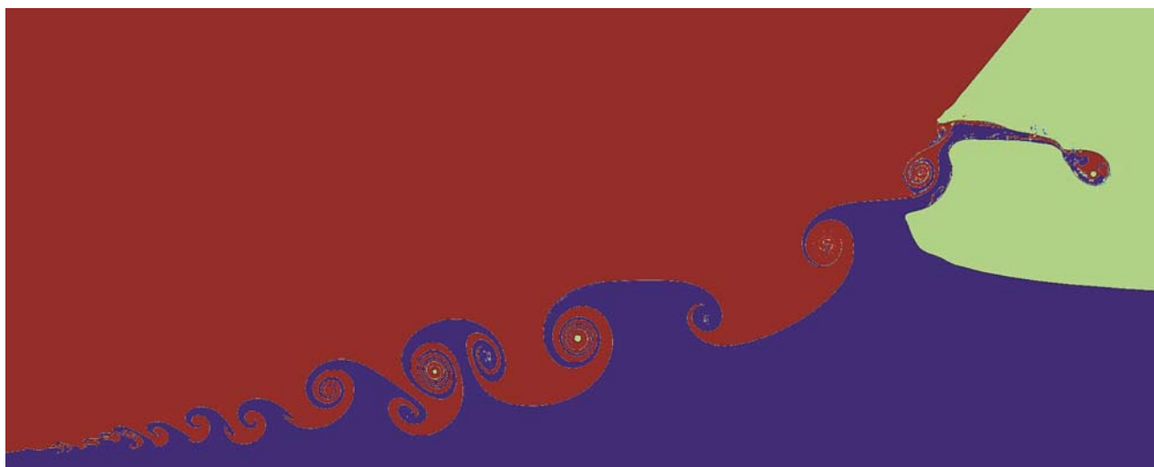
Fig. 2. Numerical simulations of the vortex street generated inside an impacting drop, similar to Thoraval et al. (2012). The red colour indicates liquid from the drop and the blue from the pool.
