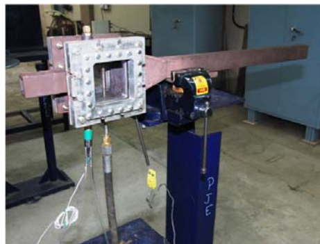
Fig. 3 Schematic of the hydrogen fuelled valveless pulsejet engine test setup and the engine mounted on the test stand.
