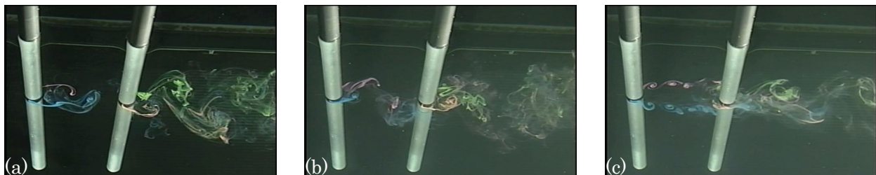
Fig. 8 Representative flow patterns in the case of distance ratio L/d=1.5 and amplitude ratio 2a/d=0.25 , (a) f/f_K=0.00 , (b) f/f_K=1.44 , (c) f/f_K=2.98
