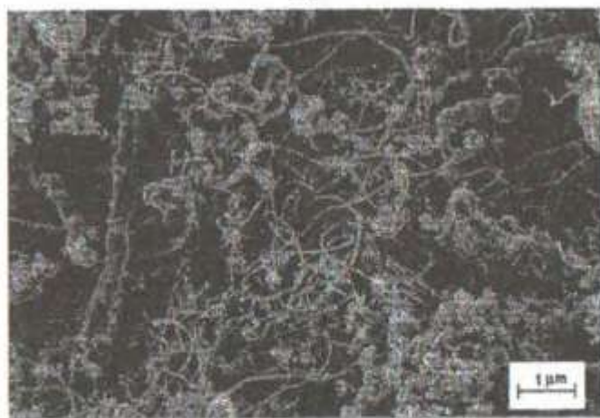
Fig. 3. SEM observations of carbon nanostructures: a – with bigger diameters; b – with smaller diameters
