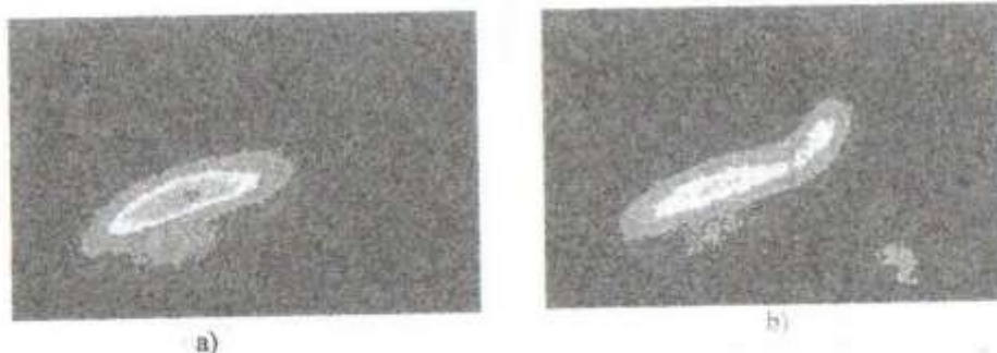
Fig. 4. Pictures of a flame without (a) and with (b) plasma obtained with optical spectral digital camera
