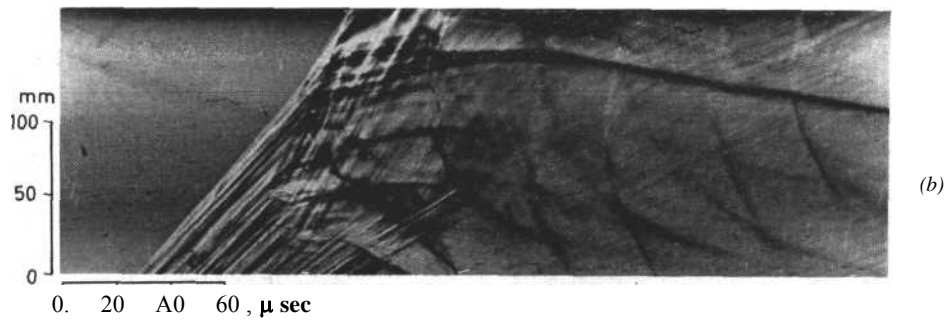
Fig. 5. Formation of detonation wave in a mixture of natural gas and oxygen
