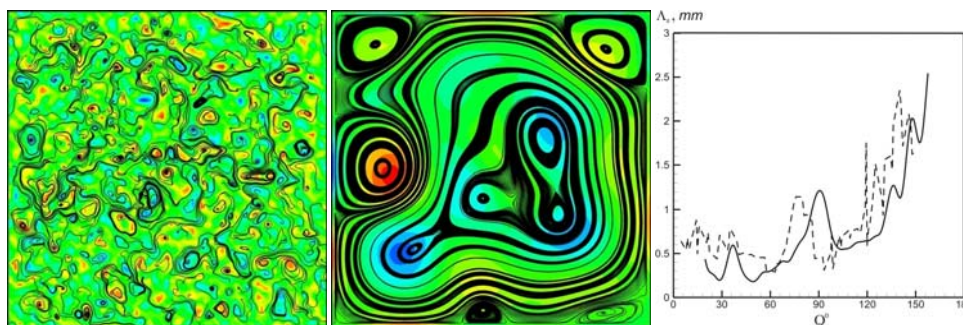
Fig. 1 Early phase of small-scale vortices birth (left). Late phase of large-scale regular structure (center). Numerical (solid) and experimental (dashed) axial component of integral length scale \Lambda_z during compression stroke, Q - crank angle (right).
