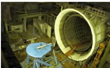
Fig. 1 Model in T-104 wind tunnel
