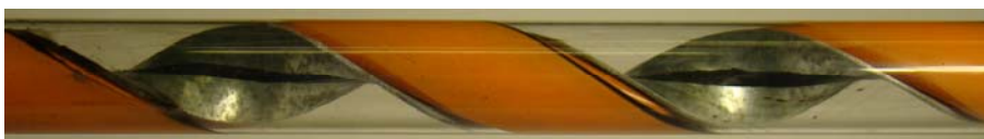
Fig. 1. The cord flow in a transparent glass tube with the twisted tape insert at big value of mass gas maintenance (the liquid is dark coloured, the one half of channel is blocked by the rubber chamber)
