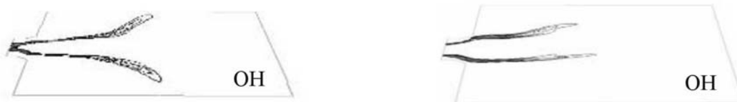
Fig. 6. OH distribution contours from the data according to Fig. 4 for comparison with case of staged air burner, in Fig. 5
