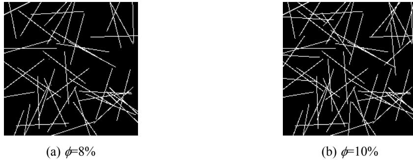
Fig. 2 Random distributed fibrous media (RDFM) generated with different fiber volume fraction, D=0.005, L=0.4
